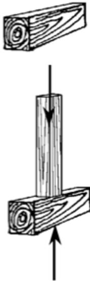
Figure 6-2. Basic configuration for vertical shores (FEMA 2014)
